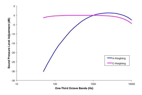
Figure 1-1: A-weighted and C-weighted Adjustment Curves
